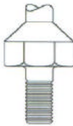
For holes countersunk on wrong side
