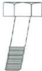
For holes which are mis-aligned
